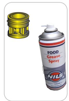
Lubricate the valve with a food grease spray
